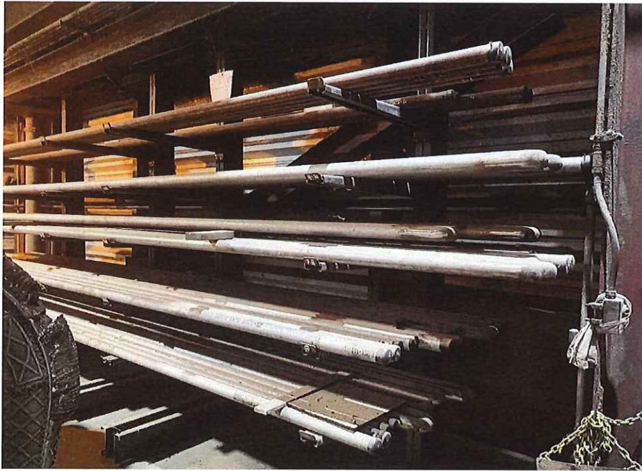
Superheater Stainless Steel Tubes
