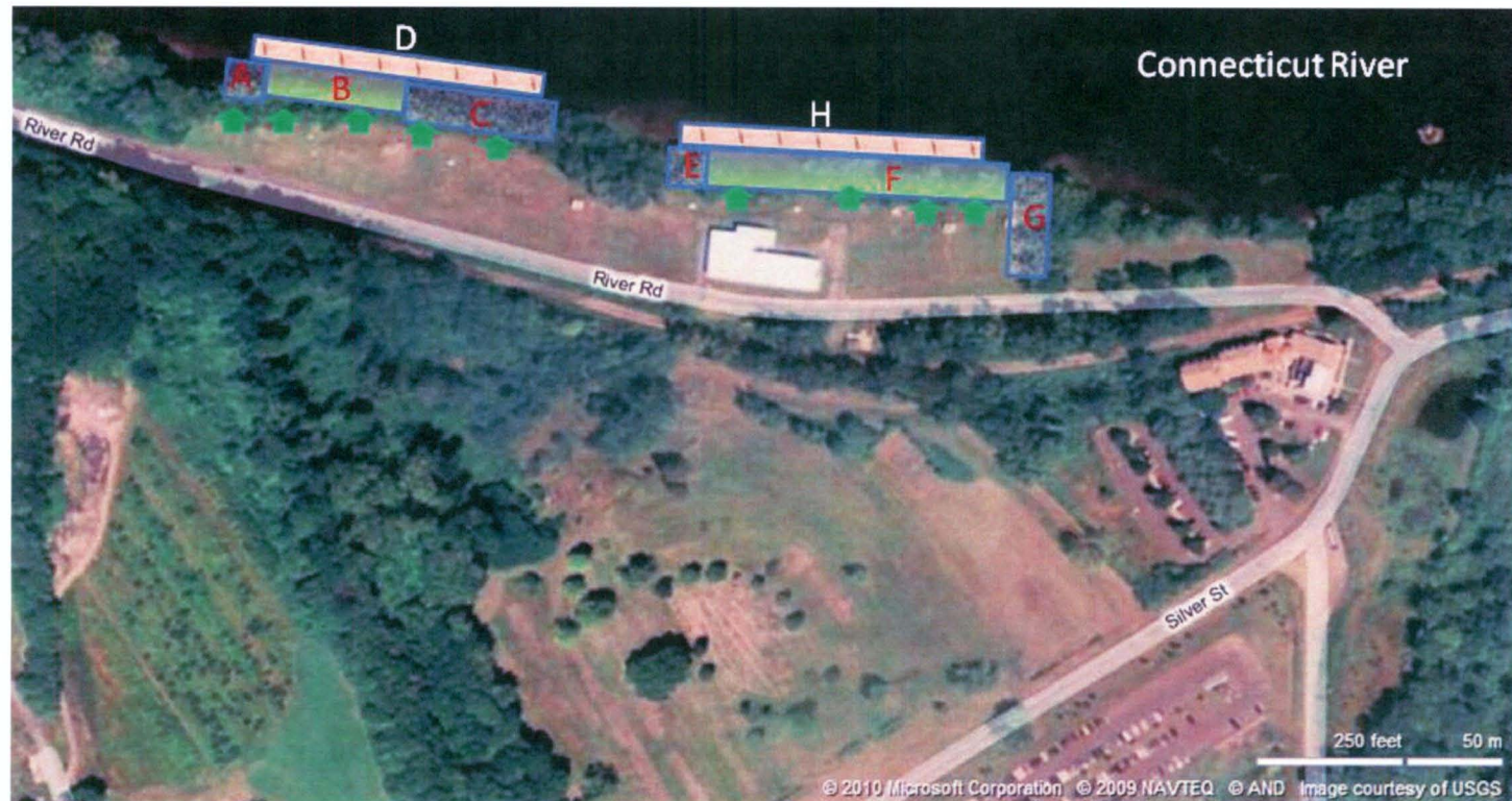
Figure 2. Proposed Design Plan for Stream bank Restoration at Middletown Well Field
